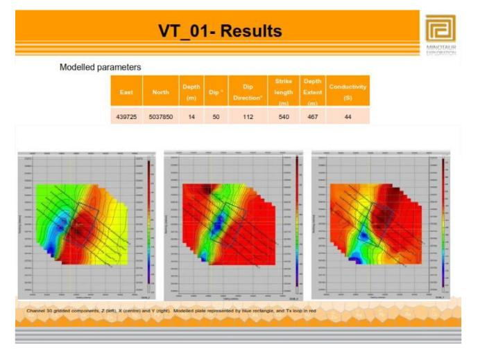
Minotaur Exploration Ltd (Australia) has confirmed the VTEM and PEM target on our BRN\_VT01 Grid at Bass River North. The body is interpreted to have a strike length of 540 meters and a depth extension of 467 meters. The target dips 50 degrees to the southeast. Both ground work and modeling suggest the target extends to the north off of the survey grid.
