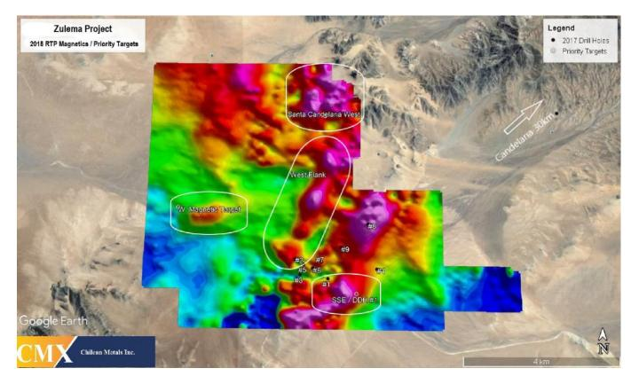
The magnetic survey delineated a 2km. wide corridor trending northeast from the southern margin of the survey area north to the Santa Candelaria workings as shown in Figure 1. A preliminary review of the data indicates there are 4 target areas that require detailed follow-up. From north to south, the targets are Santa Candelaria West, the West Flank, SW Magnetic High and SSE / DDH#1.
